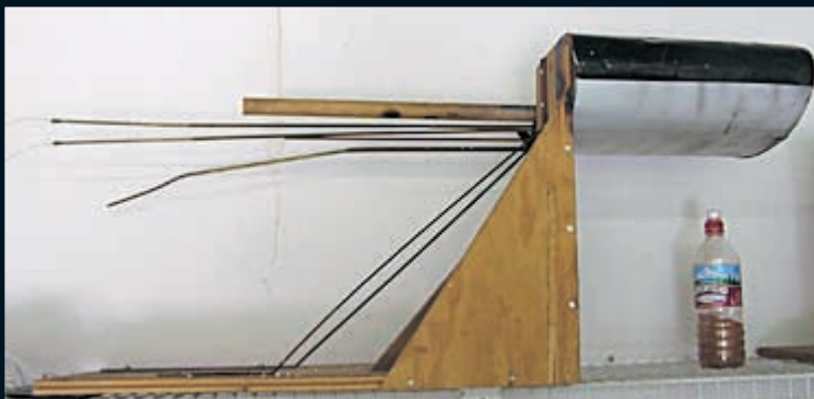
(Left): The working Chain Gun miniature operated by sliding a simple broom handle and spring wires!
